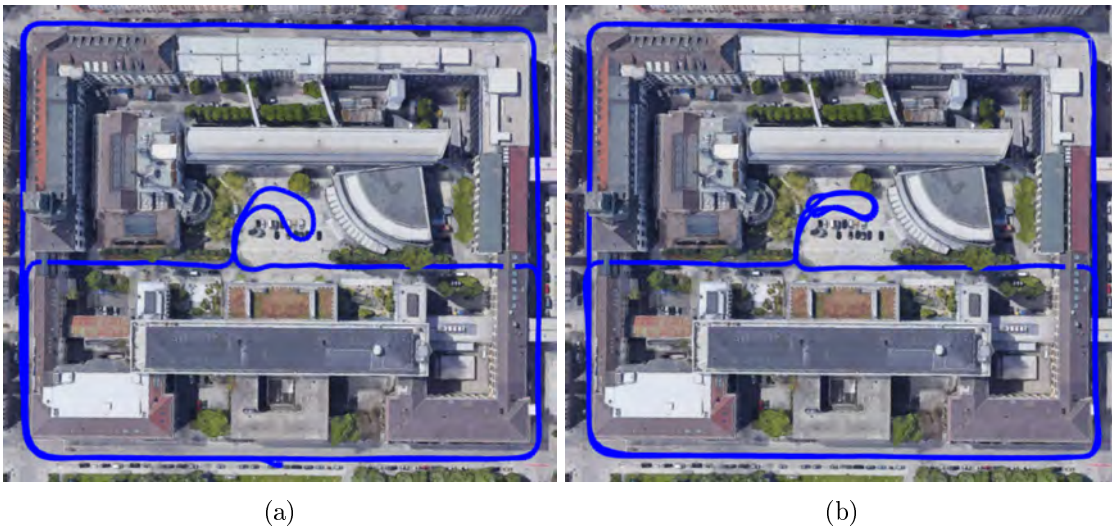
Figure 6.9: Overview of the trajectories for the TUM-MLS-2016 and TUM-MLS-2018 data set. a) Trajectory for the first data set recorded in April 2016, b) trajectory for the second data set recorded in December 2018. The source for background image and 3D model is Google Earth.
