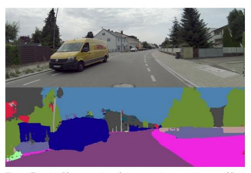
**Figure 2.** Top: original front camera image; bottom: semantic segmentation output of the given image using the ERFNet segmentation network [22].
