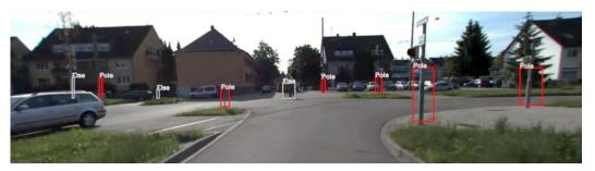
**Figure 4.** Projection of detected poles into the front camera image and classification based on the semantic segmentation image.
