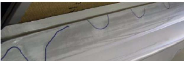
Figure 4. Defect example: waviness
