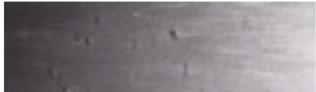
Figure 5. Defect example: pimples
