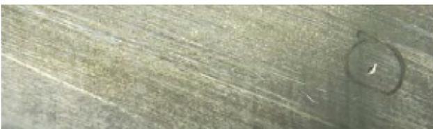
Figure 3. Defect example: notch
