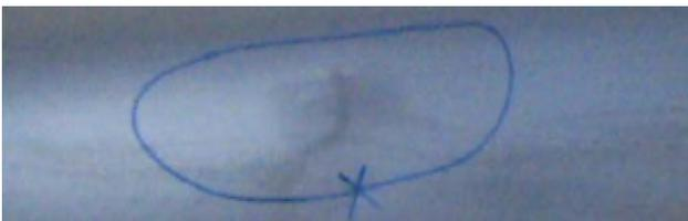
Figure 2. Defect example: bulge
