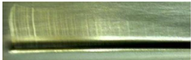
Figure 6. Defect example: scratches
