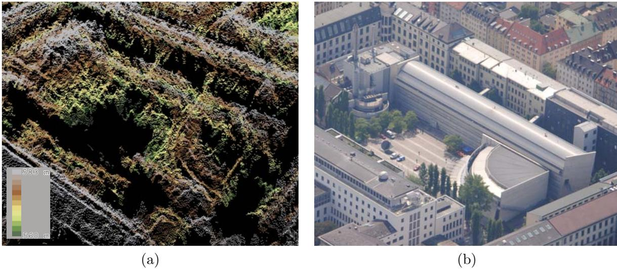
Figure 8.23: Detailed illustration of the building marked with C in Figs. 8.20 and 8.21. (a) Surface points reconstructed for the Audimax building on TUM main campus. (b) Corresponding optical image acquired during a follow-up flight campaign. Note how the curved metallic roof structures have not been reconstructed well.
