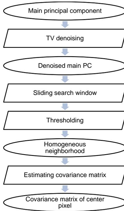
Figure 4.1: A flowchart of the PCA-TV-based covariance matrix estimation method. Note that after the thresholding an 8-connectivity check is applied.
