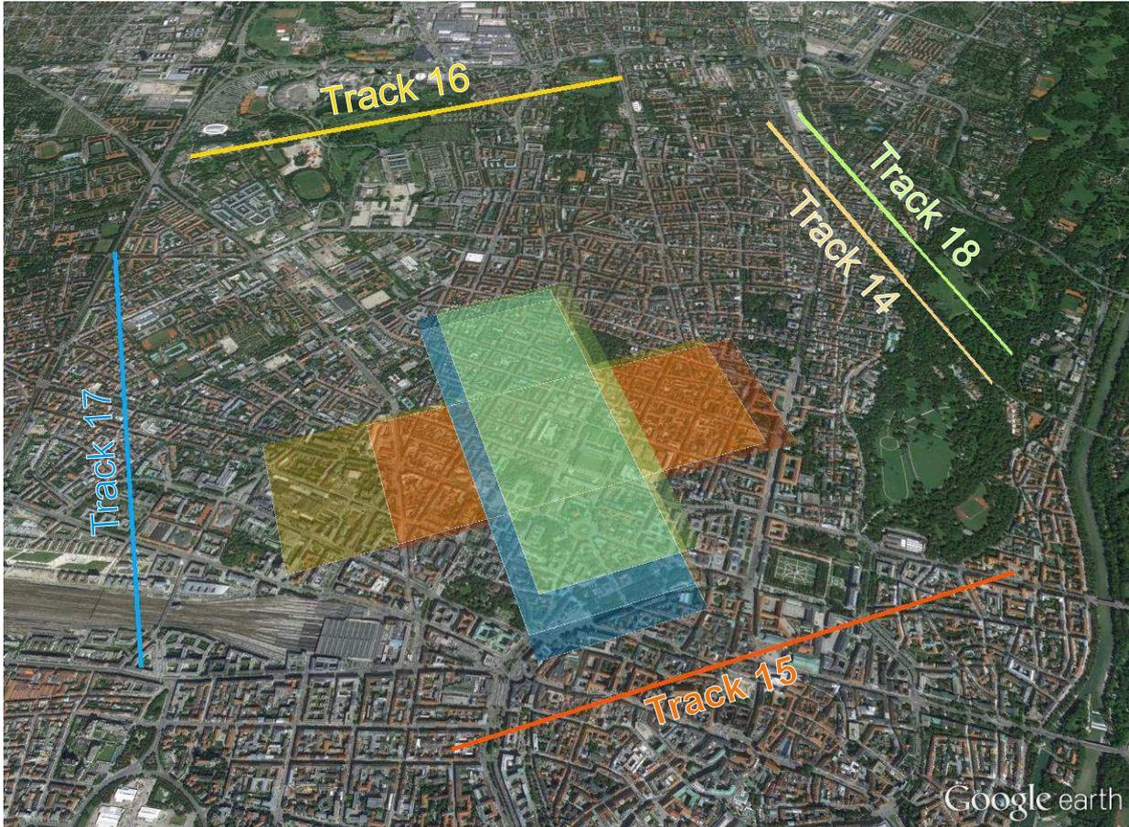
Figure 7.4: Flight track configuration and overlapping image strips of the 2011 MEMPHIS MASAR campaign (optical image of downtown Munich ©2012 Google).
