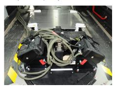
Figure 5: The 3K+ camera system. A low-cost camera system with a higher recording frequency compared to professional photographic camera systems.
