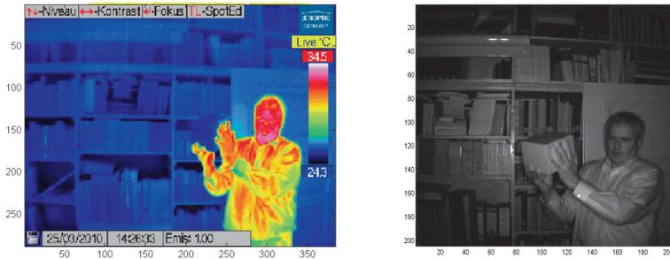
Figure 2: synchronized image pair: left: thermal infrared image with color-coded temperature, right: active intensity image of the TOF camera. Both images before distortion correction.
