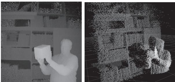
Figure 3: Left: Distance image of the TOF camera. Right: Point cloud generated from the depth image. Bright values have a smaller distance to the sensor than dark values.
