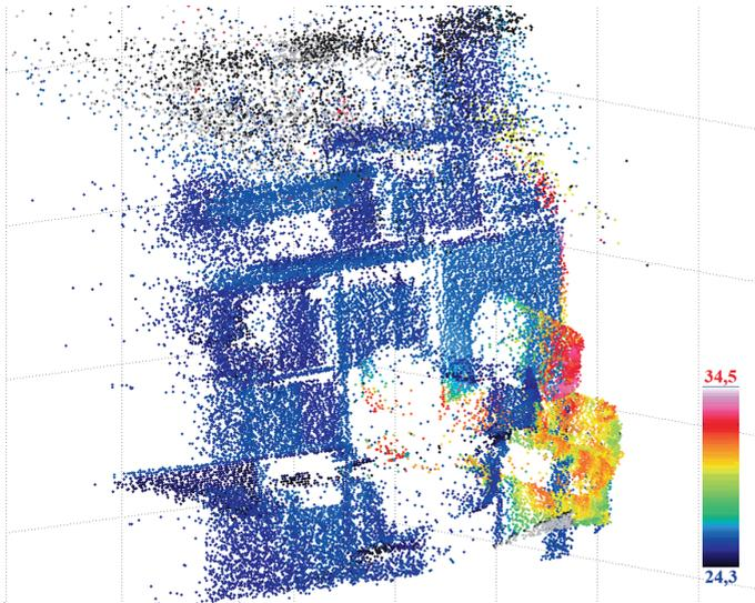
Figure 5: TOF 3d points with thermal intensities.
