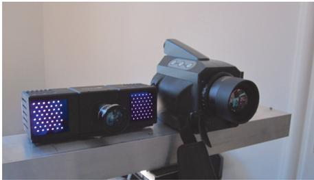
Figure 1: sensor configuration: left: TOF camera, right: thermal infrared camera
