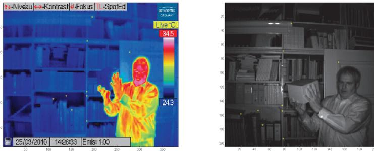
Figure 4: Same image pair as Fig. 2. Corresponding homologues points are extracted for the determination of the relative orientation.
