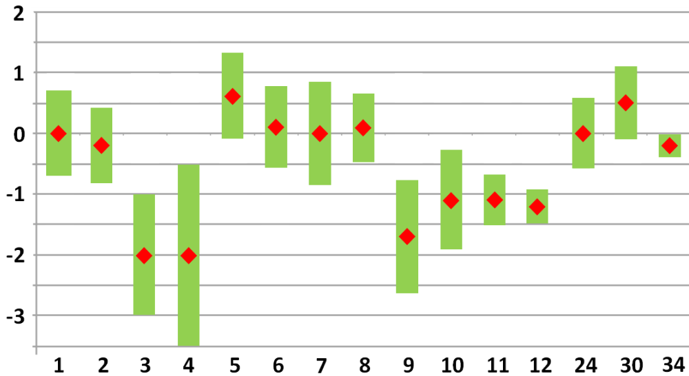
Figure 4.26.: Gable roof building height deviations : Posterior standard deviations \hat{\sigma}_b (green) and absolute differences \Delta_{b,L} to LiDAR reference (red); abscissa: only buildings where an adjustment could be conducted (more than one measured height) are shown, ordinate: deviation around the reference height in unit meter, zero corresponds to the LiDAR reference height.
