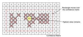
Figure 4: Suppression of multi detection
