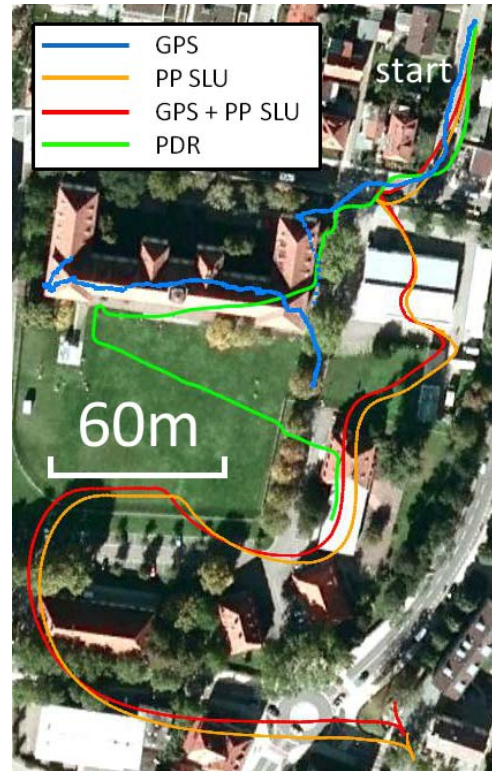
Fig. 7: Performance of PP SLU and PDR on a mixed outdoor and indoor dataset with and without GPS aiding. Results obtained with SC SLU on the same dataset are shown in Fig. 6.
