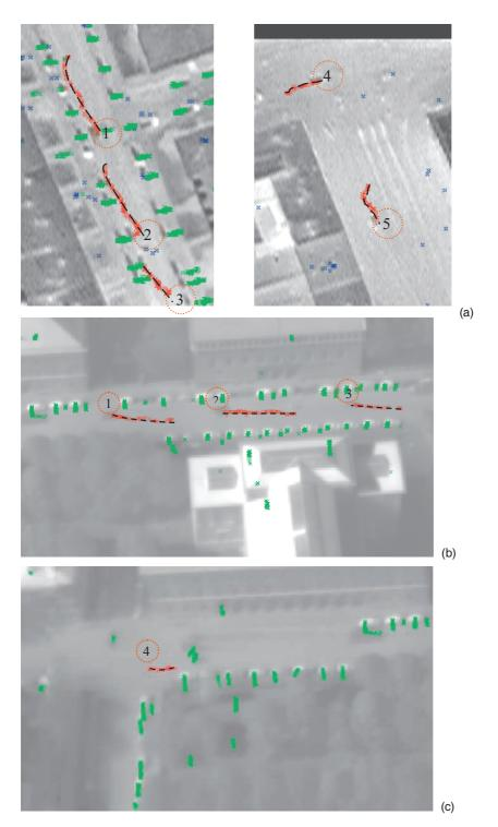
Fig. 10: Zoom into the trajectories of moving cars and their approximated curves: a) nadir-view dataset, b) and c) oblique-view dataset.
