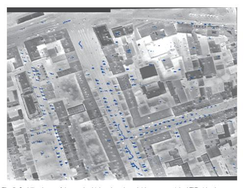
**Fig. 5:** Stabilized map of detected vehicles plotted overlaid upon mosaicked TIR video by sequential affine transformation.
