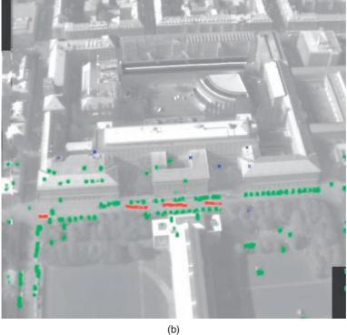
**Fig. 9:** Vehicle classification result in respect of movement: a) nadir view dataset, b) oblique-view dataset.
