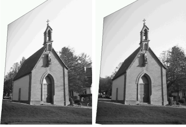
Figure 4: The first two images of Fig. 3 in epipolar geometry.
