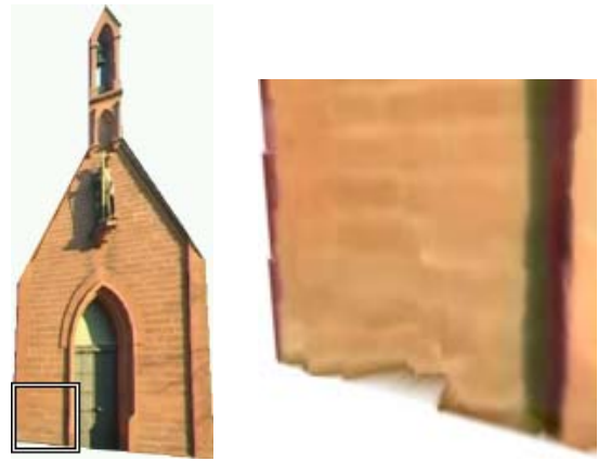
Figure 9: Gross error in reconstruction. This figure shows the lower left part of the facade.
